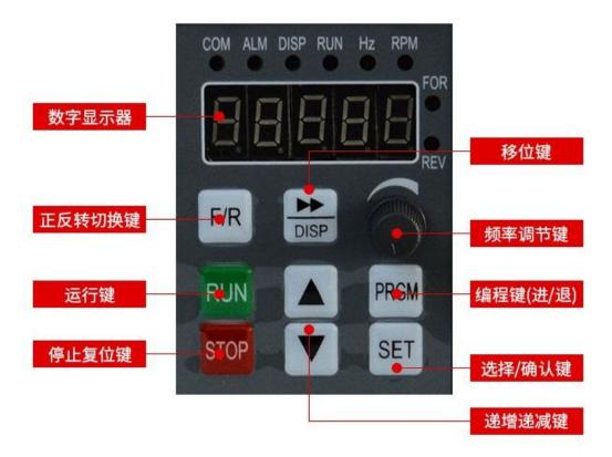
数字显示器: Digital display 正/反转切换键: Forward/reverse switch key 运行键: Run key 停止复位键: Stop reset button 移位键: Shift key 频率调节键: Frequency adjustment key 编程键(进/退): Programming key (forward/backward) 选择/确认键: Select/confirm key 递增递减键: Up and down keys
